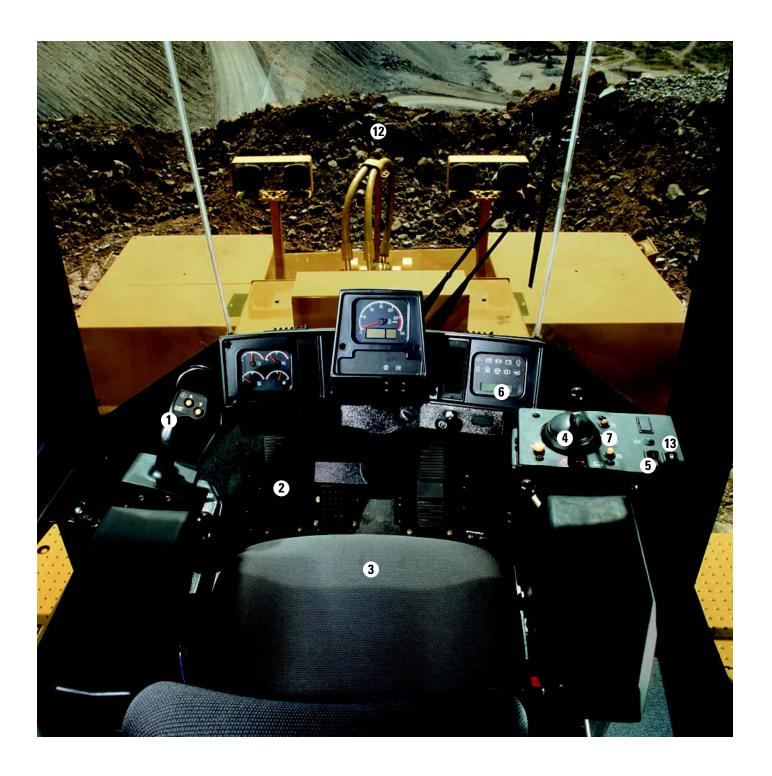
**World Class Cab.** With over 3.18 m<sup>3</sup> (112 ft<sup>3</sup>) of volume incorporates innovations for operator comfort, maneuverability and productivity. Features include outstanding viewing area, improved cab ventilation, interior sound levels below 77 dB(A), standard coat hook, cup holder, storage bin, intermittent wet-arm wipers, room for a large lunch cooler and radio-readiness.
