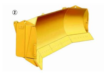
**2 Universal Blade.** Is designed for moving large loads over long distances in mining applications.
