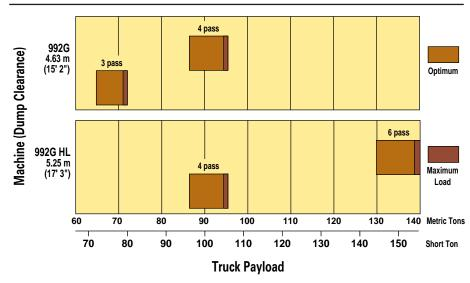
777D = 100.5 Short Ton (92 Metric Tons) maximum payload 785C = 161.1 Short Ton (146.1 Metric Tons) maximum payload
