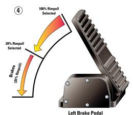
4 Impeller Clutch Torque Converter (ICTC) combined with the Rimpull Control System (RCS) allows the operator maximum flexibility in modulating rimpull.
